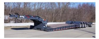
The XL Low-Profile HDG has tapered front beams, offering an extremely low load angle of only four degrees. Additionally, 42-inch flip ramps provide extra loading assistance, making it an ideal solution for the paving industry.
